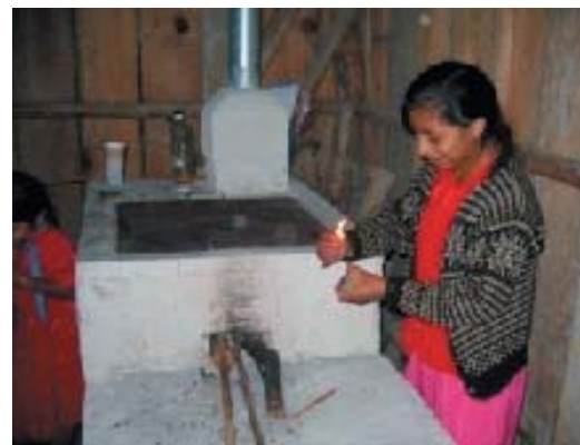
THIS ECO-FRIENDLY STOVE REDUCES ENVIRONMENTAL DEGRADATION AND HEALTH RISKS CAUSED BY SMOKE INHALATION.
